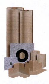
Stable substrates Laticrete's Hydro Ban Board is a lightweight construction panel designed for use in bonded tile or stone shower installations. Made with a high-density polystyrene core and waterproof cementitious coating on both sides, the boards are available in thicknesses between .25 inches and 2 inches.
