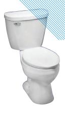
a three-bolt installation system for a sturdy, level connection between the tank and bowl. A 3-inch flush valve offers power flushing and fewer clogs, while the pilot fill valve is more consistent over a wide range of water pressures. It has an MaP rating of 1,000 grams, and complies with BAA and ARRA. 877/850-3060; www.mansfieldplumbing.com.
