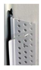
For basements, garages, and other areas where concrete walls are involved, try the new **Caulk Channel Tear Away.** The strip creates a ¼- by ³/16-inch reveal and can also be used to cover expansion areas filled with fire-rated or acoustical caulk. For use with ½-inch or ¾-inch drywall.
