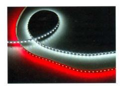
The LED Ribbon from **LED Inc.** is capable of extreme 2-axis bends and utilizes flexible-circuit technology, which allows for more applications. The product is durable, easy to use and has a high LED density for superior lighting concentration.
