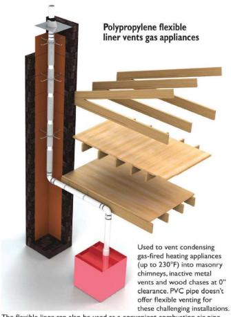
The flexible liner can also be used as a convenient combustion air pipe run to the appliance. Listed to ULC S636 venting standard. Single wall rigid pipe, fittings, adapters and flexible liner are available in diameters 2" (60mm), 3" (80mm), and 4" (100mm). POLYFLUE.
