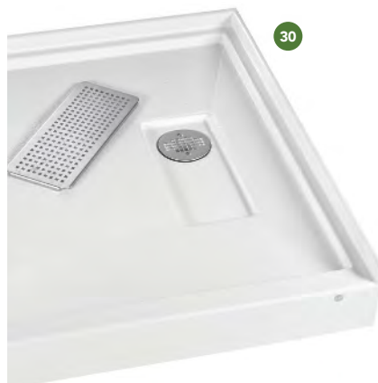
30 MTI BATHS mtibaths.com The 6036 shower base appears to be a standard model with a hidden drain at first glance until the drain cover is removed. The cover conceals an offset drain, which allows the base to replace an original narrower base or tub without repositioning plumbing. Measuring 60 in. by 36 in. and crafted from Lucite, the product is finished with multiple layers of fiberglass, resin, titanium and wood to prevent flexing. ●
